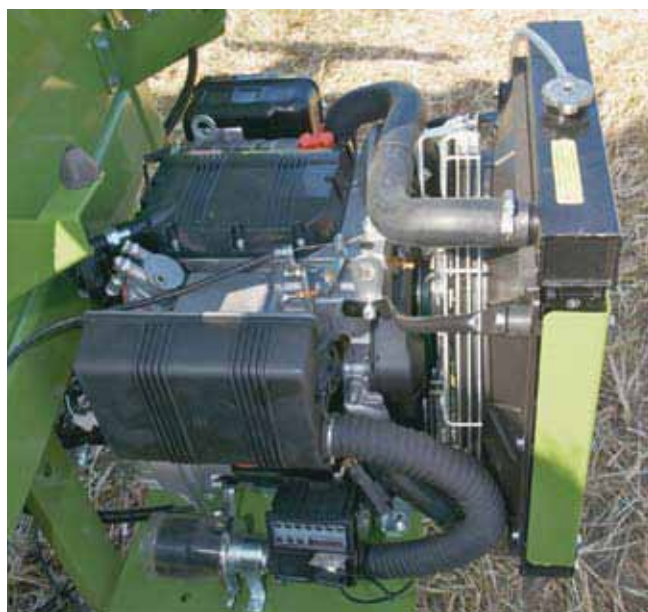
The Tube 2020 ACI has an 16 hp Lombardini diesel motor.
